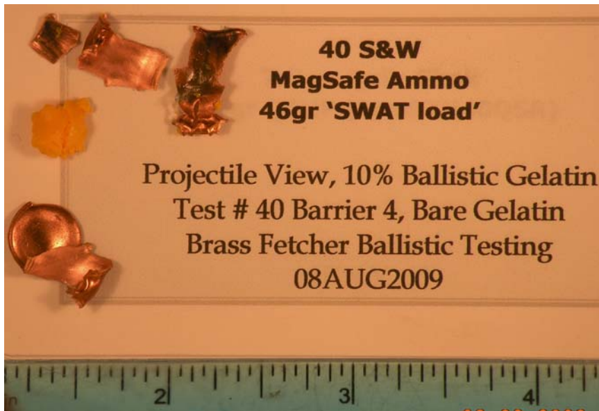
Figure 3. Projectile view of Shot 1 recovered fragments
