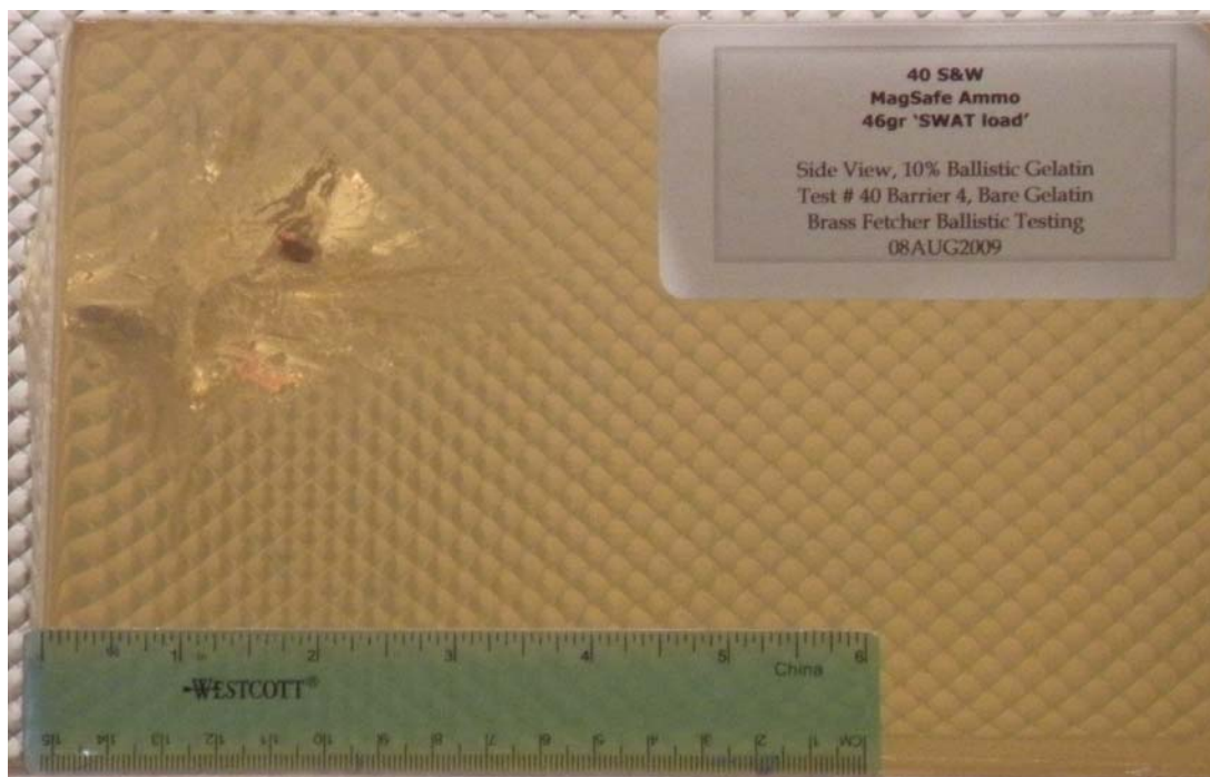
Figure 1. Side view of Shot 1 gelatin block
