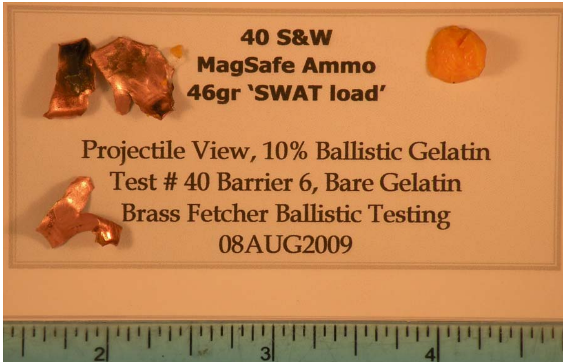
Figure 9. Projectile view of Shot 3 recovered fragments
