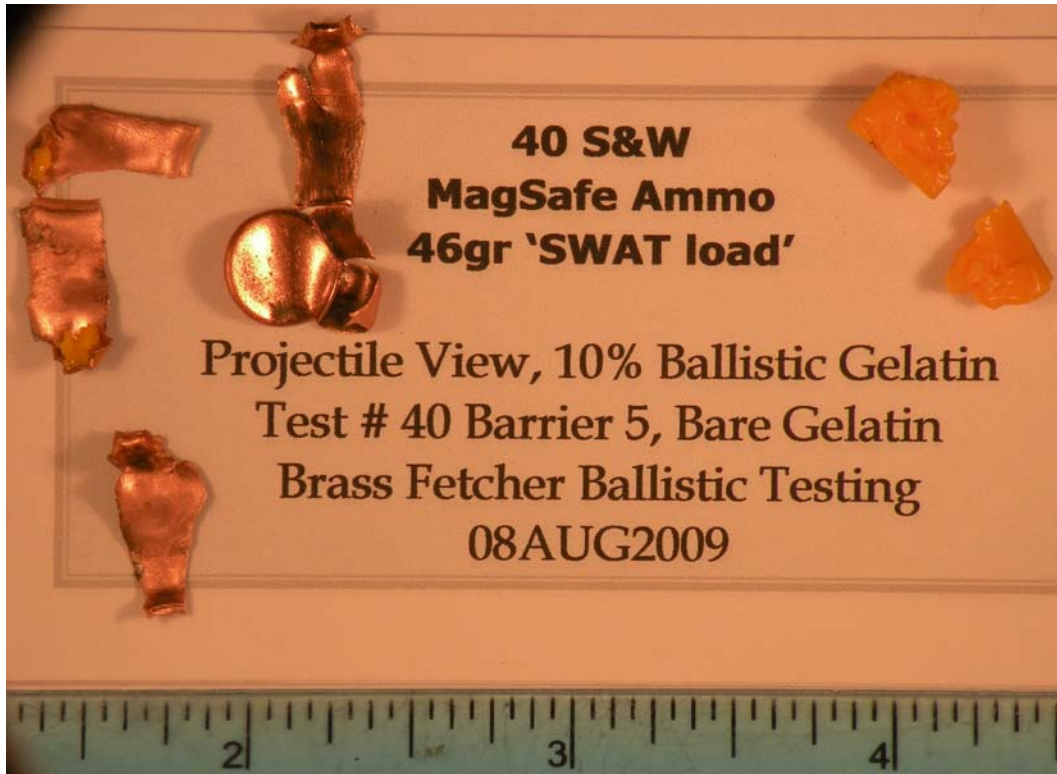
Figure 6. Projectile view of Shot 2 recovered fragments
