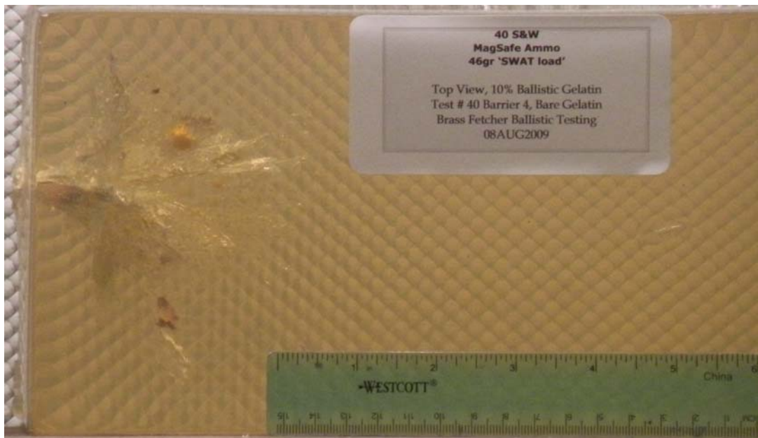
Figure 2. Top view of Shot 1 gelatin block
