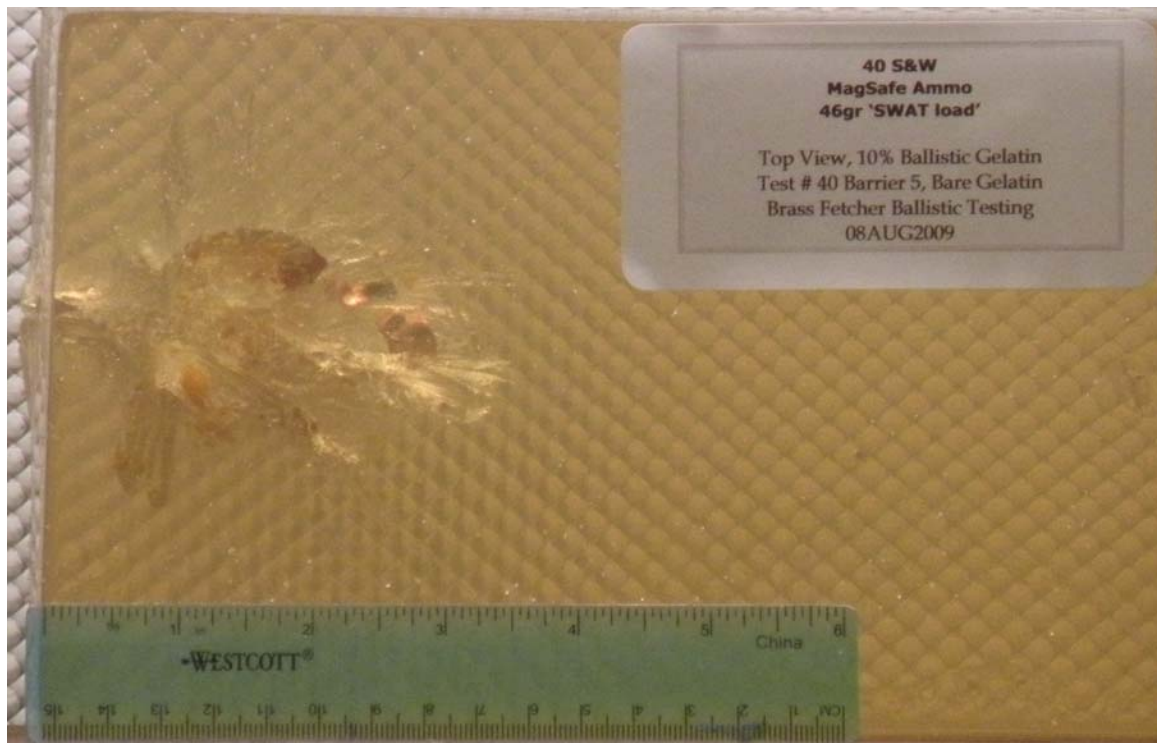
Figure 5. Top view of Shot 2 gelatin block
