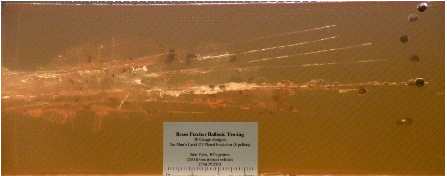
Figure 2. Side view of Shot 1 gelatin block
